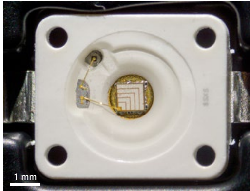
High brightness LED, chip, bond wires and packaging, Spot K LED, oblique reflected light, zoom 1.25x
