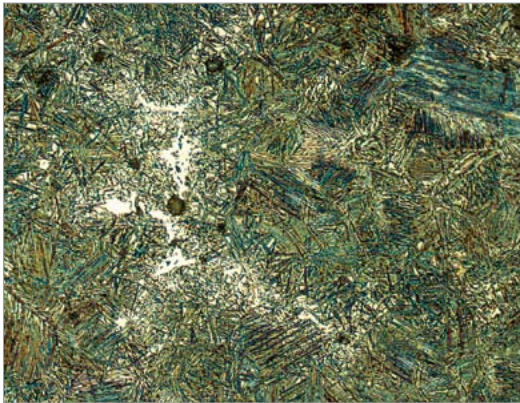
Image of an ADI sample made using a light microscope Magnification: 400:1
